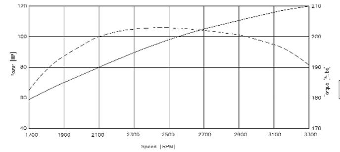
Drawing 94B4005/1 3300 ENGINE POWER CURVE
